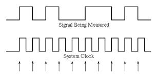
The rising edge of a clock signal from the circuit being tested is used to measure and display other signals from the system.
