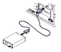
3. Turn the emulation probe's power switch ON. Power is supplied by the module/probe interconnect cable.
