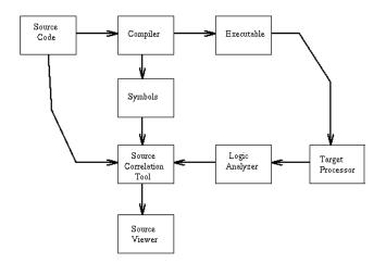
Source code is written by the designer and compiled into an executable while creating a by-product symbol file. The executable is downloaded to run on the target processor, and the symbol file is loaded into the
